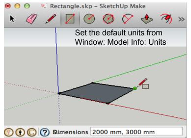
Start by drawing a rectangle (R) and type in the X and Y dimensions.
