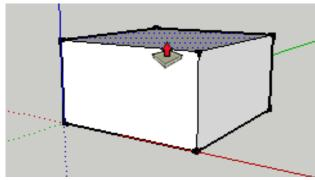
Click on the top surface with the Offset tool (F) and drag out.
